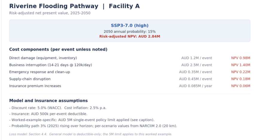
Figure 3 Worked per-pathway financial model for the riverine flooding pathway under the SSP3-7.0 scenario, Facility A. The worked example applies the facility's actual AUD 5M single-event policy limit; the general loss model in Section 4.4 is deductible-only.
